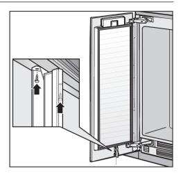
Screw the air separator to the middle of the appliance door using two screws.
